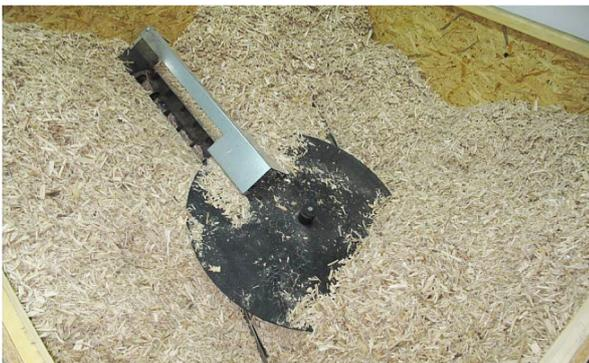
Wood chip storage with the mixer connected to the transporter
