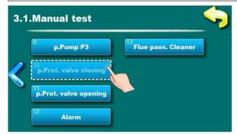
Option for protection valve (closing) test.
