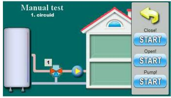
Option for testing elements of 1st heating circuit (mixing valve (START-open), mixing valve (START-ope
