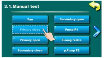
Option for primary air motor device (close direction) test.
