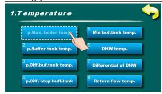
In this parameter is possible to adjust maximal boiler working temperature.
