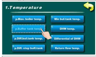
In this parameter is possible to adjust buffer tank temperature.
