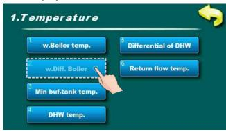
In this parameter is possible to adjust difference of boiler working temperature.
