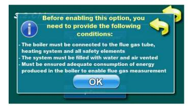
This option allows the flue gas measurement.
