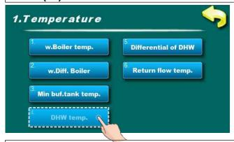
In this parameter is possible to adjust domestic hot water temperature.
