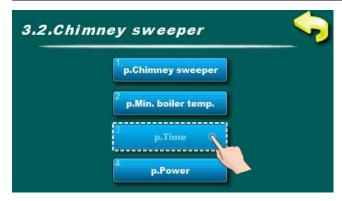
In this parameter is possible to adjust time for flue gas measure.
