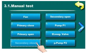
Option for secondary air motor device (close direction) test.
