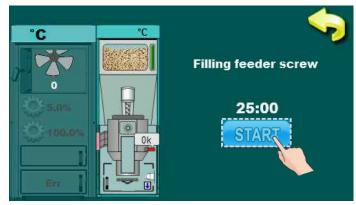
This option allow filling of empty feeder screw with pellets. At start-up or missing fuel, when is feedery screw empty this option is used for filling feeder screw. By pressing "START" feeder screw start with work. This option must be turned on until fuel start droping from feeder screw.
