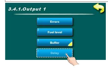
This parameter define after how long will be again activate error / warning of fuel level / low temperature of buffer tank (this parameter doesn't work if is selected continous signal).
