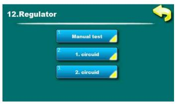
Menu "Regulator" is showed only if module for two heating circuits CM2K-B is installed and configurated.
