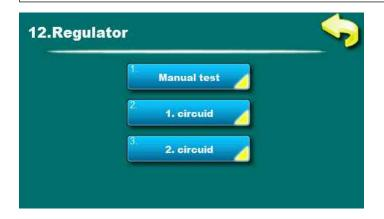
Menu "Regulator" is showed only if module for two heating circuits CM2K-B is installed and configurated.
