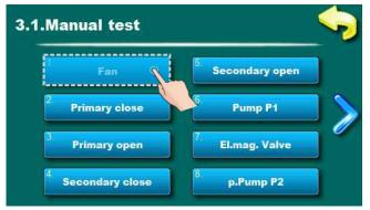
Option for boiler fan testing.
