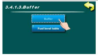
This parameter define whether will it output 1 report warning for low temperature in buffer tank. This option don't allow setting of his own table for signal type in different time of day, but adjusted table for fuel level warning can be used. For using table for low temperature in buffer tank is neccessary to activate table for fuel level (see Figure below).
