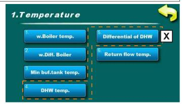
**X** - only if "**DHW**" (domestic hot water) exist on heating system (must be configured like additional equipment)
