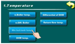
In this parameter is possible to adjust minimal buffer tank temperature.
