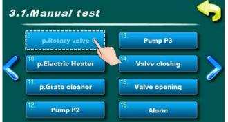
Option for backfire protection rotating valve (RSE) test.
