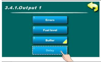
This parameter define after how long will be again activate error / warning of fuel level / low temperature of buffer tank (this parameter doesn't work if is selected continous signal).
