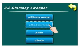
In this parameter is possible to adjust minimal boiler temperature at flue gas measurement.
