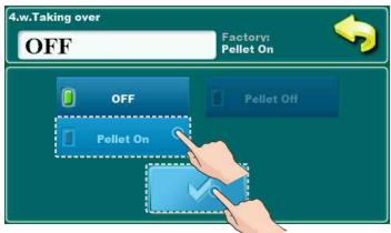
On main menu (menu: WOOD(w)) (see Point "8.1.4. Main menu") choose submenu "4. Taking over", select "Pellet On" and confirm it by pressing "Confirm" button.
