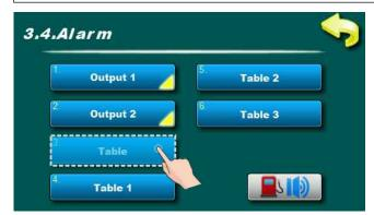
This parameter is used to select the predefined table for the alarm. The automatic switching on and off or changing the signal type at a specific time. It is possible to adjust signal type for speaker and signal type for low fuel level warning. The table will be operational only if is "table" selected in point 5.7.9.1 for output 1 (signal type).
