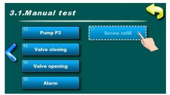
Option for pellet feeding system test.
