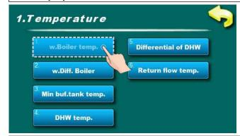
In this parameter is possible to adjust boiler working temperature.
