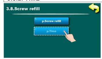
In this parameter is possible to adjust how long will be work option for feeder screw fill.
