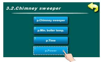
In this parameter is possible to adjust boiler power for flue gas measurement.
