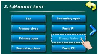
Option for electro-magnetic valve test.
