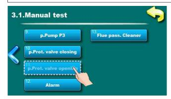
Option for protection valve (opening) test.
