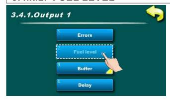
This parameter determines whether the output 1 fuel level warning occur. By selecting certain types of signals will be activated in the selected signal format.
