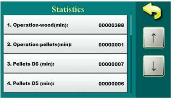
The regulation follows the startup number of the boiler and the work time of certain parts of the boiler.
