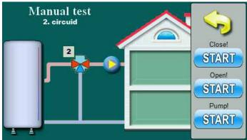
Option for testing elements of 1st heating circuit (mixing valve (START-open), mixing valve (START-close) and pump (START)).
