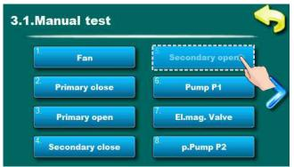
Option for secondary air motor device (open direction) test.
