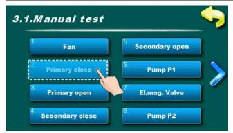
Option for primary air motor device (close direction) test.
