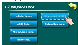
In this parameter is possible to adjust difference of domestic hot water temperature.
