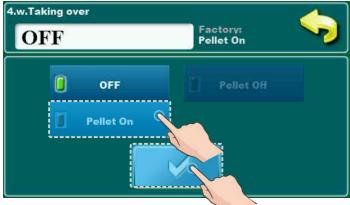
On main menu (menu: WOOD(w)) choose submenu "4. Taking over", select "Pellet On" and confirm it by pressing "Confirm" button.
