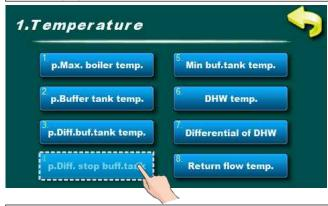
In this parameter is possible to adjust difference of buffer tank stop temperature (condition for boiler shut down and pause).
