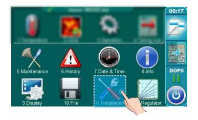
This menu can use only authorized persons. For entry in "Installation" menu is necessary to input PIN.
