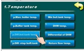
In this parameter is possible to adjust difference of buffer tank temperature.
