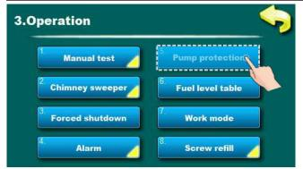
In this parameter is possible to enable /disable pump protection.
