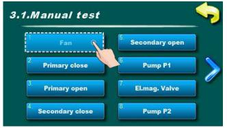
Option for boiler fan testing.
