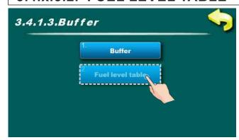
In this parameter is possible to turn on / off table for fuel level alarm.
