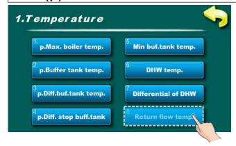
In this parameter is possible to adjust return flow temperature.
