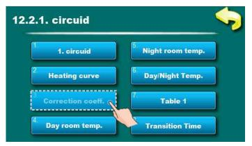
This parameter determines the influence of the room corrector. When this coefficient is larger, room corrector will more affect to the calculated required flow temperature in the heating circuit.
